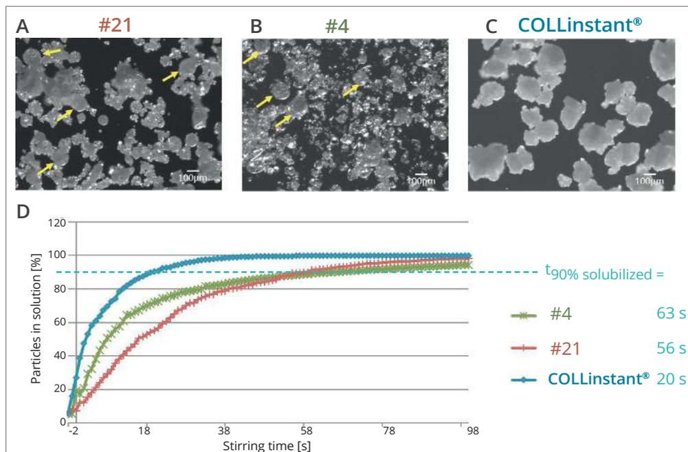
**FIG 7:** Microscopic analysis of competitor collagen hydrolysate agglomerated powders (A, B) and COLLinstant® (C).
