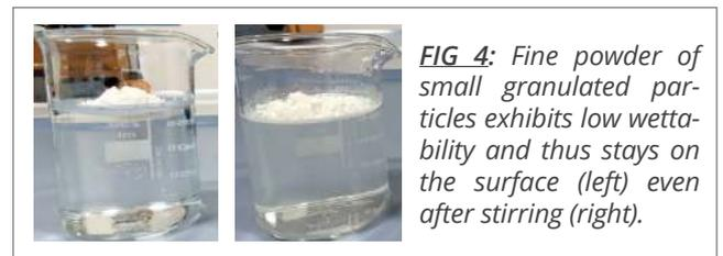
FIG 4: Fine powder of small granulated particles exhibits low wettability and thus stays on the surface (left) even after stirring (right).
