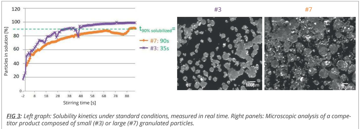
FIG 3: Left graph: Solubility kinetics under standard conditions, measured in real time. Right panels: Microscopic analysis of a competitor product composed of small (#3) or large (#7) granulated particles.
